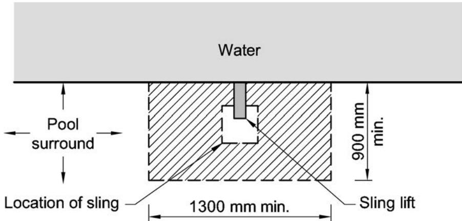
**Diagram b. Clear space for sling lift in the transfer position**
